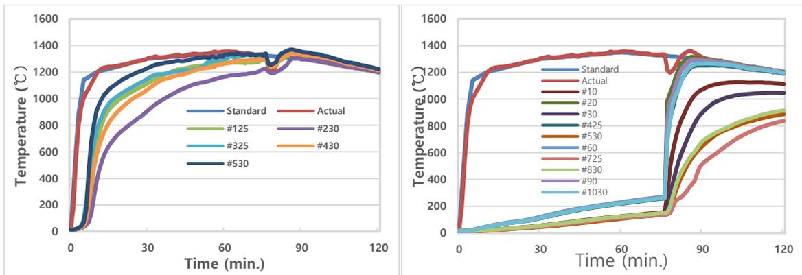
**Fig. 5** Time-Temperature Curves for RWS : Reference (L) and Fire-protected (R)
