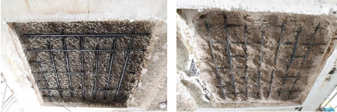
**Fig. 7** Spalling of RC Slab for RWS : Reference(L) and Fire-protected(R)
