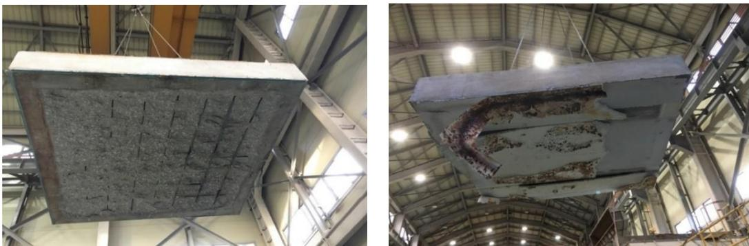
**Fig. 6** Spalling of RC Slab for RWS : Reference(L) and Fire-protected(R)
