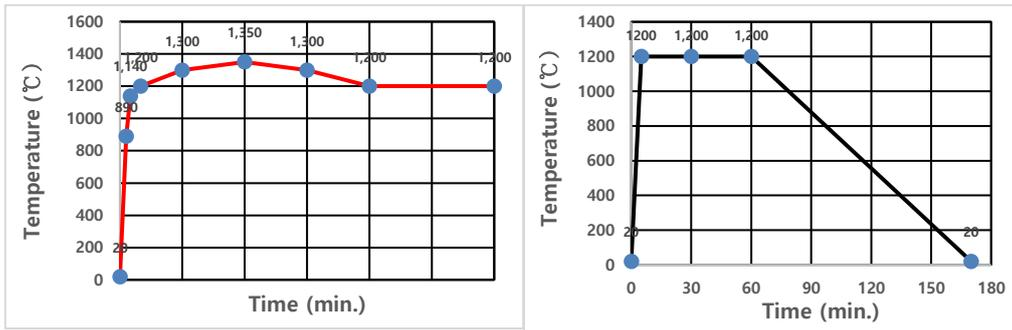
※ Two curves have been used to imitate tanker fire in Netherland and Germany, respectively.
