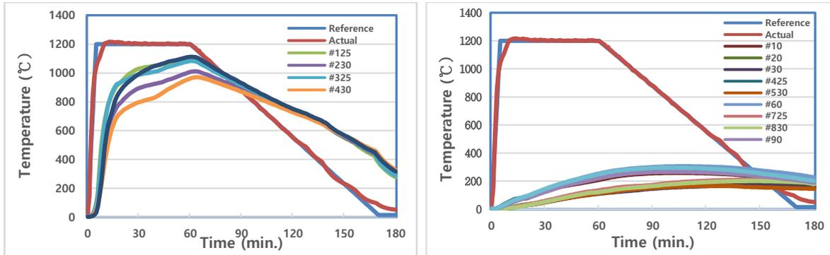
**Fig. 4** Time-Temperature Curves for RABT : Reference (L) and Fire-protected (R)
